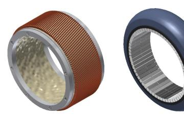
Windings: Litz wire wound diagonally around a 3D printed mold.
